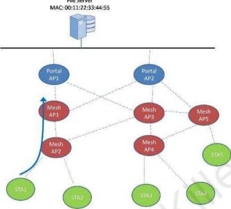
STA1 sent a data frame to Mesh AP2 destined for a local file server on the same subnet with MAC address 00:11:22:33:44:55. Mesh AP2's mesh forwarding algorithm determined that the frame should be forwarded through Mesh AP1.In the frame sent from Mesh AP2 to Mesh AP1, what is true of the contents of the MAC header? (Choose 3)
