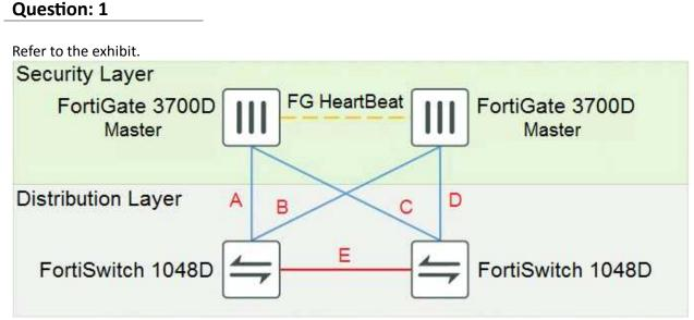
The exhibit shows a full-mesh topology between FortiGate and FortiSwitch devices. To deploy this configuration, two requirements must be met:
