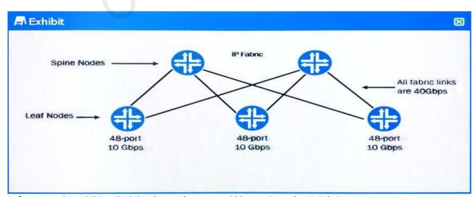
Referring to the exhibit, which hardware change would be made to the IP Fabric to ensure an exact
