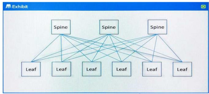
A customer has a 3-stage Clos architecture with three spine devices as shown in the exhibit. If a single spine device fails, what percentage of the remaining bandwidth will be available from leaf node to leaf node?
