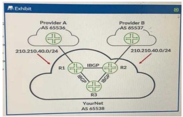
YourNet is learning the 210.210.40.0/24 route from Provider A and Provider B YourNet would like to forward traffic destined to the 210.210.40.0/24 networking using Provider B. Referring to the exhibit, how would you accomplish this task?
