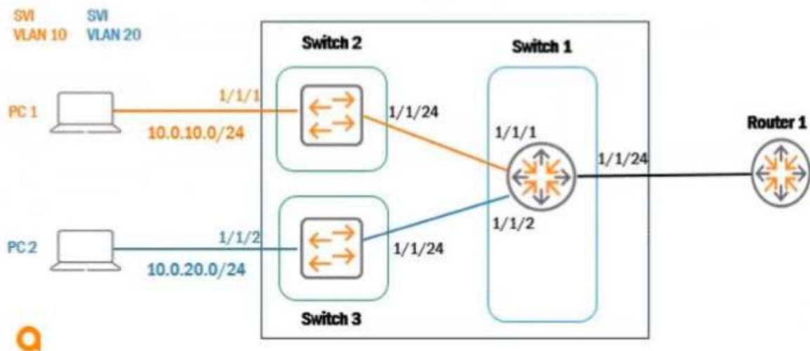
Based on the given topology, what is the requirement on an Aruba switch to enable LLDP messages to be received by Switch 1 port 1/1/24. when Router 1 is enabled with LLDP?
