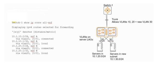
You are adding a VLAN 30, subnet 10.0.30.0/24 to the network shown in the exhibit. (This network is simplified to just the relevant switches for this item.) This subnet belongs in VRF A, and you have added a Layer 3 VLAN 30 interface attached to this VRF on Switch-1. You want to make the services in this VLAN available to devices in 10.1.20.0/24 in VRF B.
