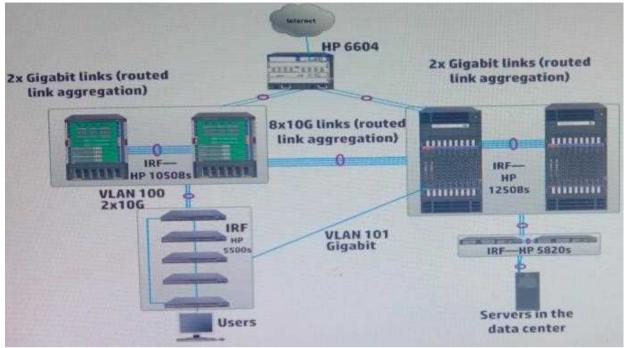
The exhibit shows the topology for an enterprise LAN with an on-site data center. The intelligent Resilient Framework (IRF) group of HP 5500 Series switches supports a group of computers that require very high availability to the data center. Therefore, the customer has requested a backup gigabit fiber link implement Open Shortest Path First (OSPF) in a single area.
