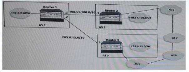
These three routers are currently configured for BGP. They do not apply any routing policy in terms of BGP on routers or attributes advertised to an received from peers. How can the network administrator for Router 1 cause Router 1 to advertise 192.0.2.0/24 to Router 2 and Router 3?
