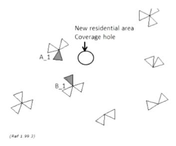
A new residential area has recently been built showing a lack of 3G uplink coverage as shown in the exhibit. The terrain is flat and all the buildings in the area are 20 meters in height with no other relevant direct obstacles. What should be applied to cells A\_I and 8\_1 to provide 3G service to the new area knowing that both cells have a soft handover (SHO) factor of 1.9?
