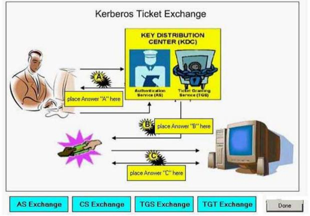
In a Kerberos Ticket Exchange, three exchanges are involved when the client initially accesses a server resource. As shown in the diagram, label each of the three exchanges.
