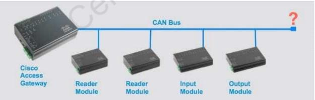
One or more expansion modules is connected to the Cisco Access Gateway via a CAN bus. How should the CAN bus wires be connected after the last module in the chain?
