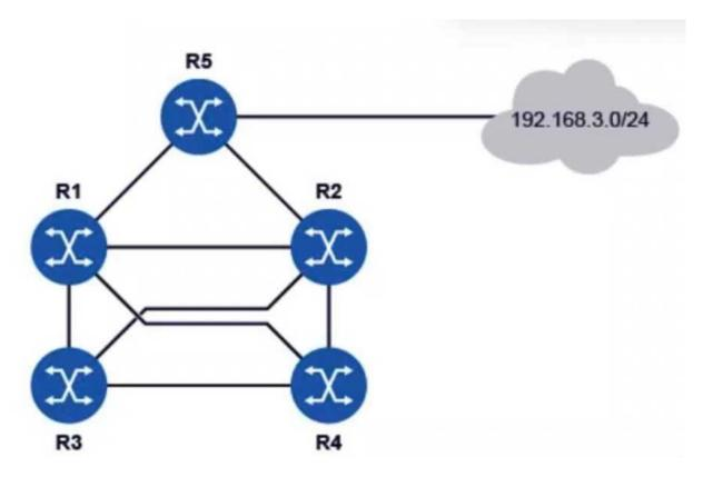
All routers in the diagram are running an interior gateway protocol (IGP) and have been configured with an ECMP value of 4. Router R5 advertises the prefix 192.168.3.0/24 using the IGP. Assuming all links have the same cost, how many entries for prefix 192.168.3.0/24 will be in router R3's routing table?
