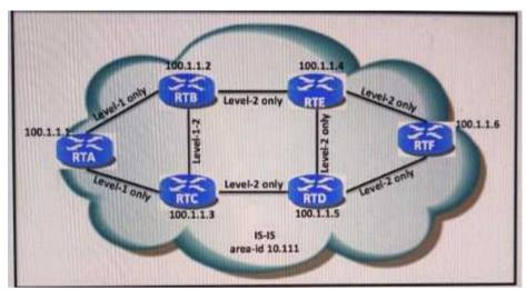
Refer to the exhibit. There is reachability among all routers. An MPLS TE auto-tunnel mesh is deployed in all routers. A full mesh auto-tunnel is created successfully among RTB, RTC, RTE, RTD, and RTF routers. RTA router is able to build an automatic MPLS TE tunnel that has only RTB and RTC routers as destinations. Why is the RTA router unable to build an automatic MPLS TE tunnel that has RTE, RTD, or RTF routers as destinations?
