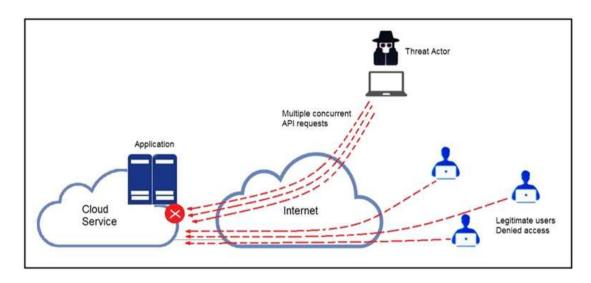
A threat actor behind a single computer exploited a cloud-based application by sending multiple concurrent API requests. These requests made the application unresponsive. Which solution protects the application from being overloaded and ensures more equitable application access across the end-user community?
