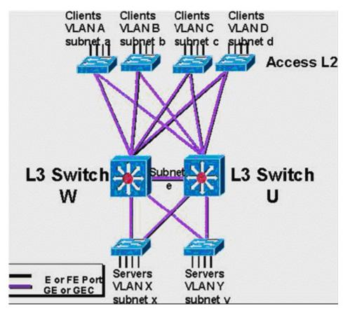
The diagram shows a collapsed L3 switched building backbone consisting of two L3 switches: W and U. Each L3 switch has a routed interface on every subnet (VLAN) in the building. There are no VLAN trunks in the network. In other words the L3 switches are acting as native routers. There are exactly 4 client-side VLANs (subnets): a, b, c, d. There are exactly 2 server-side VLANs (subnets): x and y.
