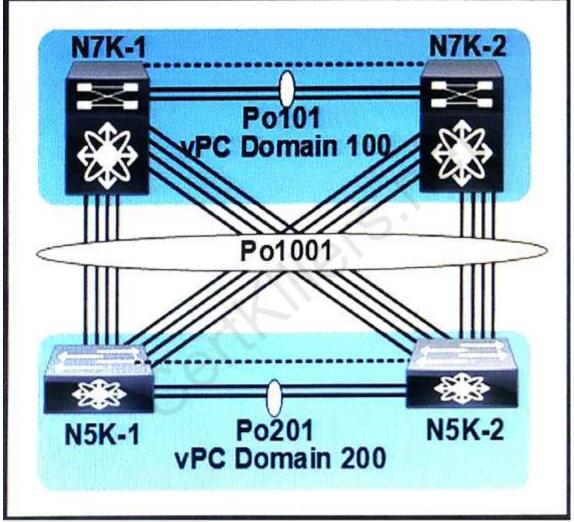
You must ensure that the vPC Domain 100 controls the LACP Po1001 link. Which feature do you configure?
