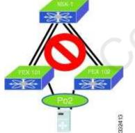
If you need to connect a multi-homing server to a pair of FEXs when there is only one Cisco Nexus 5000 Series device, you have the option to run active or standby NIC teaming from the server. Reference:
