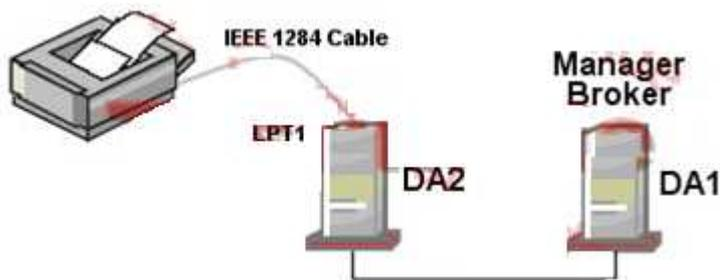
You need to configure a special purpose thermal-transfer printer for your organization. Because it doesn't have a built-in network interface, you've connected it to LPT1 on your DA2 server using a parallel cable. The Printer Agents for your organization's printers are managed by an iPrint Manager and Broker on your DA1 server. You want to configure the iPrint Manager on DA1 to manage this new printer as well. Will this configuration work?
